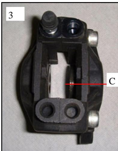
3. With a tool narrow enough to fit between the disc and caliper (e.g a screw driver) push the pistons ( C ) back until there is room to slide the pads in ( 1 each side )
